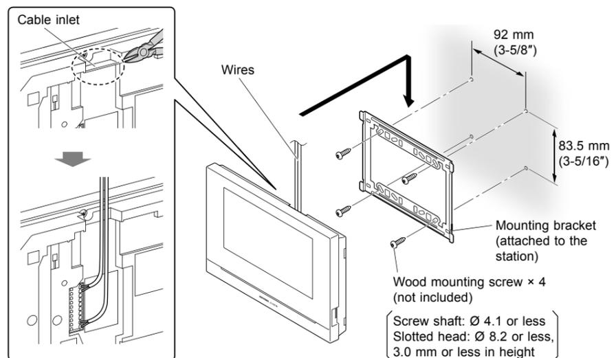
When wood mounting screws cannot be used for plasterboard walls, concrete walls and so on, use commercially-available board anchors or concrete plugs.
