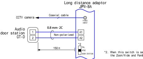
\*2. When this switch is set to either "NTSC" or "PAL", the Zoom/Wide and Pan&Tilt functions are disabled.
