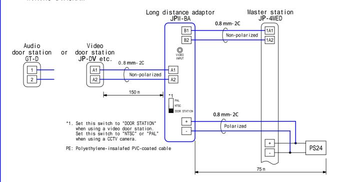
· Connecting a CCTV camera and an audio door station in place of a video door station
