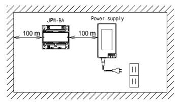
Locate JPW-BA together with Power supply inside an Enclosure box or other protected for limited access.
