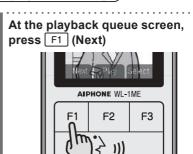
The first image of the previous record will be displayed. When displaying the oldest record and pressing, the display will return to the latest recording.
