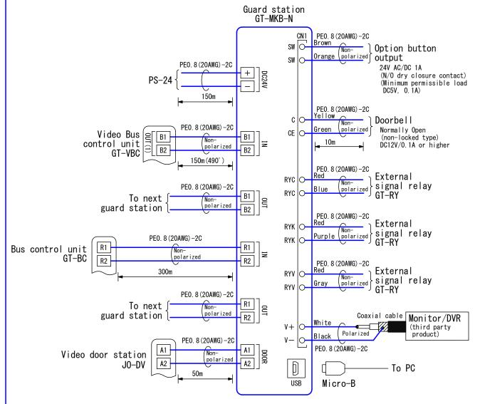
PE: Polyethylene-insulated PVC jacket cable
