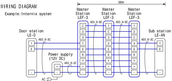
Wiring may vary according to combination of Master & Sub stations.
